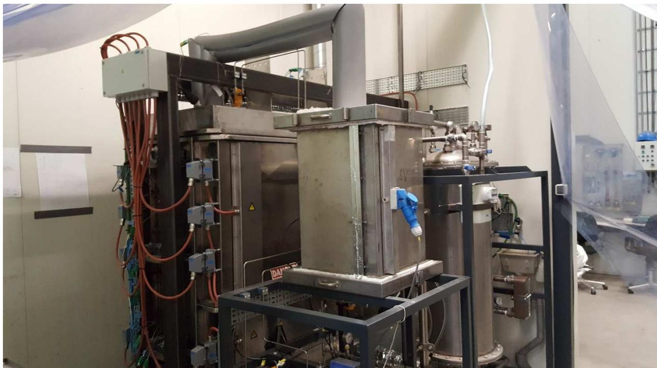
**Fig. 2:** Photograph of the autothermal catalytic reformer (~2 kg/h) in the BTG laboratory.
