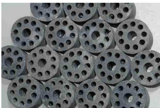
**Fig. 4:** Steam reforming catalyst used in the gasifier
