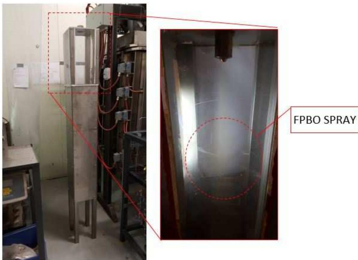
**Fig. 5:** Photograph of the atomization investigation setup.
