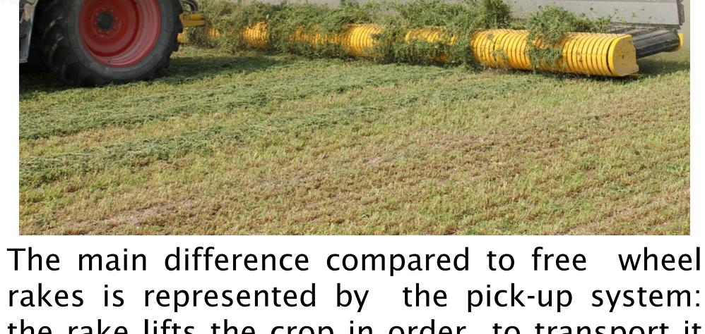
rakes is represented by the pick-up system: the rake lifts the crop in order to transport it on a conveyor belt, whereas traditional rakes drag the crop on the ground up to the windrow. This difference leads to:
