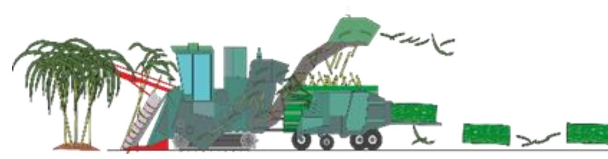
A big baler without pick up and feeded directly by the discharge system of the sugar cane harvester that is blowing the dry leaves will be towed by the harvesting machine. The top leaves discharged by the topper and the straw discharged from the second fan will be directed into the soil, as normally happens. This approach will not collect any soil and stone, will decrease the field traffic and the damage of the roots by avoiding the windrowing and pick up for baling operations.
