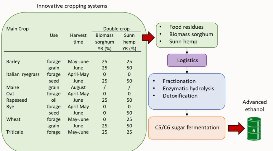
Figure 1. Value chain overview starting from innovative cropping systems (main crop + double crop) feedstocks until the final advanced bioethanol production.
